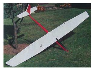
First design published was in the Jan. '69 issue of Flying Models. It had a hatch/power pod combo that interchanged with a separate hatch for slope/tow. It could fly 3 ways and was dubbed the TRI-BELLE. Wing was built up, 100" span.
