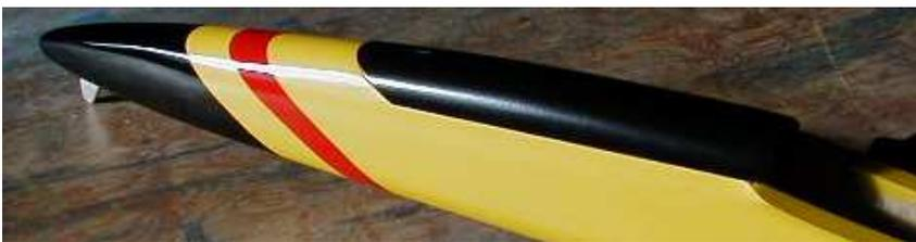
**Fins are 5/16" light balsa with internal bell crank. Light spackle fillets at the tail make the fuse, fin & skid look one-piece.**
