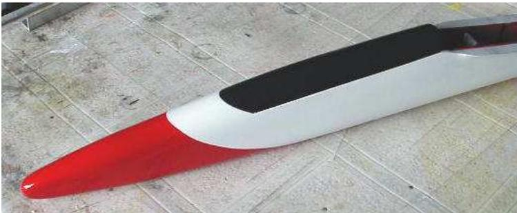
**All feature well-secured one-piece nose blocks to drill out for a lead shot/resin mix. Molded glass canopies come with the parts packages. All have removable, single tooth nose skids made of 1/8" aluminum. Fuse cross sections by the fin are small, but strongly reinforced with CF laminate under ply doublers.**
