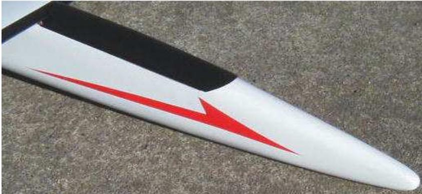
**All slim, curvy fuses/fin may be inexpensively scratch-built with glass cloth, birch ply, balsa, a little CF laminate & adhesives. They are known for their beauty, durability & finish. The lower right pic has perspective distortion, but displays the prominent droop snoot-bowed boom configuration. Modelers are startled to learn they are not expensive molded creations.**
