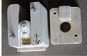
Glue sides to the bottom to snugly fit servo case. True up rear end so a plate can be glued there to butt servo against. Drill a 3/8" hole in top piece, cut a bit oversize. Center hole over output gear, mark and trim top.
