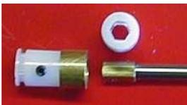
The 3/8" x 5/8" coupler with its single set screw is shown with a partially inserted adapter, set screw, brass reinforcing sleeve for heavy duty applications and the 3/16" x 3/8" hex end of a drive shaft. Nicely squared up, tap the set screw hole with a 4-40 tap or any longer 4-40 screw.
