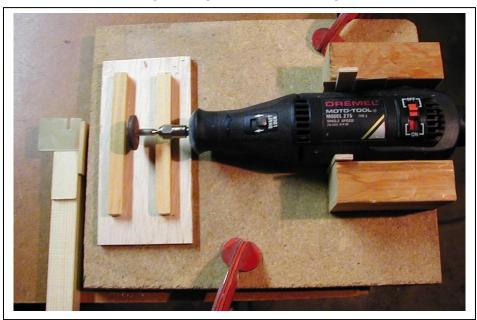
To a ¾" base, glue a ½" thick platform. Snugly support the Dremel between glued-on blocks. Stabilize with shims or attach a metal strap over it. Optionally, blocks can also be glued either side up front to further stabilize it. Note the tool can still be shifted laterally. This enables positioning the cutting disk in
