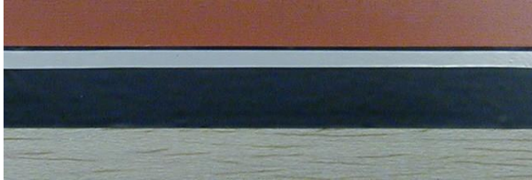
This shows \frac{1}{8} " tape over \frac{3}{4} " tape stuck to the balsa fuse side by the canopy opening. Note \frac{1}{32} " clearance. Ignore the brown background.
