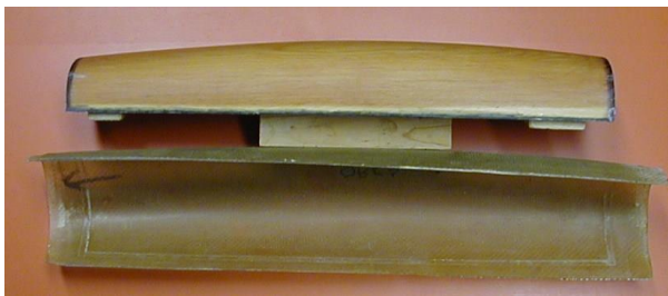
This shows the '89 ORCA plug & mold. After shaping fuse top (with plug), the plug is removed & ends are extended \frac{1}{8} " for trim tape where black stain is seen. Note trim lines formed inside mold by the \frac{1}{8} " tape. used. Black stain lines indicate where tape was once affixed.
