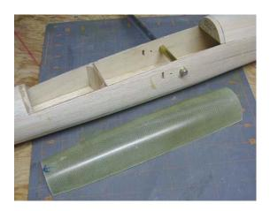
Trim the glass canopy to its molded-in reference lines. Out of the mold, it may widen or narrow. Make pliable with heat gun. Squeeze between blocks to narrow. Press to widen. The 1/8" balsa fuse doublers are contoured to SS outer edges to make oval-like cross sections along entire fuse. Tape canopy in place. Merge fuse lines to it. On balsa sheet, mark inside canopy to outline end supports. Cut & glue on as this pic illustrates.
