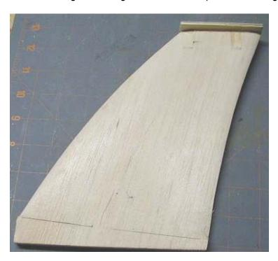
Later, after mostly shaping the fuselage, sand fin areas above the SS top edges to sort of a generic, symmetrical airfoil without flat spots. From a layer of 1/16" balsa & 1/16" ply, make the platform with bolt holes aligned to the brass inserts. Epoxy platform in place, squared-up, balsa side down. Strength & rigidity are later imparted in filleting & glassing-over. The bass stab blocks referred to below can be seen installed at the top of the fin under the stab platform.
