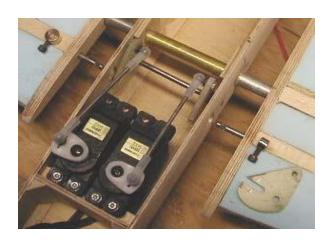
Panels, fitted with 11/32" brass tubes, rotate on a 5/16" steel rod. 1/8" drive pins, notched for wheel collar setscrews, protrude to enter slots in cams (lower right) that pivot on a 1/8" wire shaft across the fuselage. Servos & cams, shimmed with washers to clear the sides, are fitted with 2-56 ball links. Pushrods are all-thread 2-56 steel. At their rears, servos mount on a 1/8" ply crosspiece secured to side rails. See next picture.
