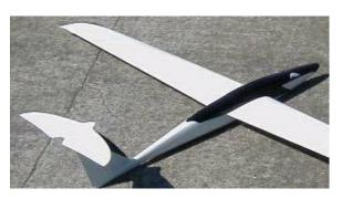
This new wing has equal LE & TE sweep. Pivoting at 45% of chord, the aerodynamic balancing makes lighter work for servos. The new Mark Drela airfoil combo optimizes overall performance & handling.
