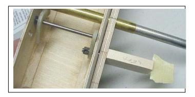
Measure how much pin should protrude to eliminate play between endcap & fuselage.
