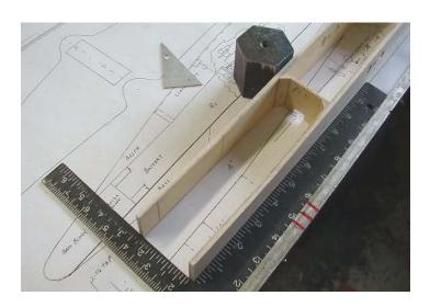
Review next picture about TS. To attach the fuse left side, position the work upright as shown here. Use a carpenter's square to align the front ends. Use weights or clamps to keep things together as glue dries. Keep flush to the workbench from 0" to 14" to align sides in profile.
