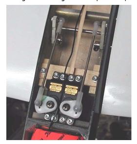
JR 368 BB micro digitals are shown here & above. Output arms need to be rigid & sturdy. Wheels, trimmed for clearance, are used. If ballasting is intended, lead blocks or stacks of lead sheet can be attached to the fuselage floor. See BALLASTING, page 14. Linkages need to be slop-free. Secure ball links with provided nuts. Apply CA glue around nuts.
