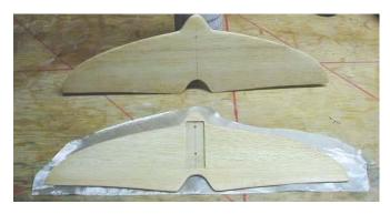
The top picture shows the 1/32" ply core glued to the 1/8" bottom, edges trimmed to core. Next, the 1/8" top has been glued on, & all surfaces gently rounded, ready for glassing-over. To top side, brush glass down smoothly & wrap it around the edge & over the bottom a little. Sop excess resin. Let this cure, sand bottom glass edges smooth, & then size a glass piece to fit the bottom & brush it down. Sop excess. When cured, sand the overlaps smooth.
