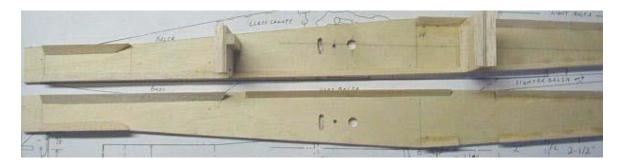
Forward of the fin, the TS is to be trimmed to allow clamping it between the SS's. Preferably, use solid 5/16" very light sheet balsa for the fin. 3/8" is overkill.  $\frac{1}{4}$ " is too thin for the threaded inserts. Alternatively with 3M77, laminate light 1/8" balsa sides to a 1/16" light balsa center.
