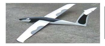
The '89 version TE sweep looked racy, but extra area behind the wing pivot point made hard work for the servos at higher speeds.
