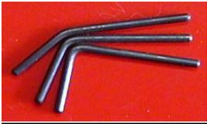
PRE-BENT WIPERS are \$5 a pair in .104" STANDARD (wire size 37) and .1285" HEAVY DUTY (wire size 30) diameters. These are machine bent from 2-1/4" lengths of precision, flat ground, polished steel drill rod stock, then hardened and tempered. Short arm is .75" long.
