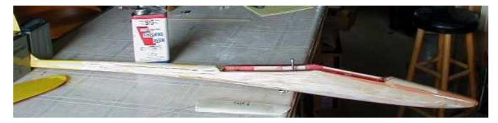
The fuse was first masked to repaint the interior red. Then this was shielded with cardboard to spray yellow on the horizontal edges where the canopy and wing go. Then overall yellow was applied to the main fuselage.
