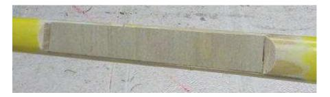
New balsa was added to the 1/64" ply. The "Icing" putty mentioned in the Fine Finishing file was used to fill creases, pits and dings on the exterior.
