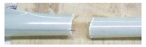
I removed the pushrod pieces and rejoined them with a metal split sleeve. By making a small hole in the skid area of the fin, the rear coupler could be visually aligned and threaded back into the bell crank clevis after the fuse was repaired.
