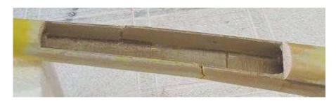
Each of the three doublers was sized to make full contact with existing structure. The rear ends were beveled to prevent rudder cables from catching on them when later inserted forward from the exit holes by the fin.
