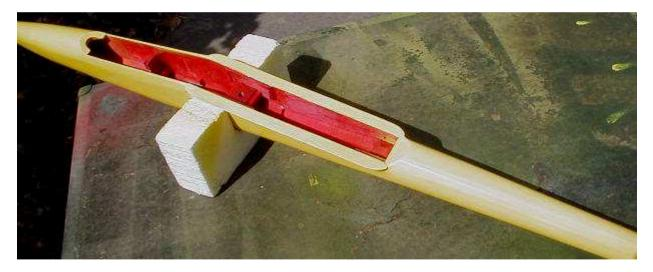
The restored fuse looks like new and is stronger than it was originally. The repair can't be found. Using a hacksaw and files, a hook tooth was made from a piece of aluminum T-bar to screw attach under the nose. Servos are in, new canopy fine-fitted and painted. Rudder cables and pushrod are hooked up, ready to fly.
