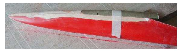
The lcing putty was used to fill a dip forward of the canopy where I cut too deeply.
