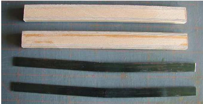
Initially, make these boxes with 1/8" thick tops & bottoms. Add to the **bottom** to get to web height. Mark which is the **top**. After dividing the box at its center, the **outboard** half along its **bottom** can be tapered toward its outboard end. See pics on pg. 8. When jacking up the center section to set dihedral between Sec. 1 & 2, this tapering **optionally allows a bit more dihedral** before the outer box end pokes out of Sec. 2.
