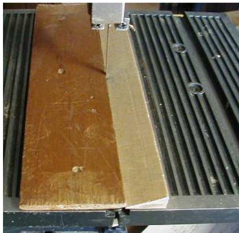
Little down aileron is needed for turn. TE camber for launch requires more. Tilt bandsaw table or tape a beveled support to it. Against the blade, clamp a board. Experiment with a 5/16” sq. strip of balsa to learn how to make the bevel. Bear the inverted aileron on the support & against the board to bevel it without taking anything off the top skin. Finish up with sanding blocks.
