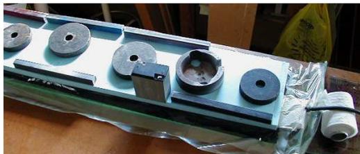
Put the beds outside of the bag with the carriers properly positioned between. Weight down & draw vacuum. Keep the work in a warm environment for the recommended time & preferably longer so the TE’s are rigid & not subject to warping when out of the carriers. Aileron warps will especially cause unwanted turning tendencies.
