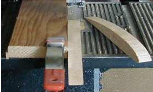
Here, with bandsaw table not tilted, a 1/8" x 3/8" strip (extreme left) has been attached to the edge of a 3-1/2" board to tilt it 1/8". The guides for the blade should be set to prevent blade wobble. Use a sharp blade or a straight line cannot be cut.
