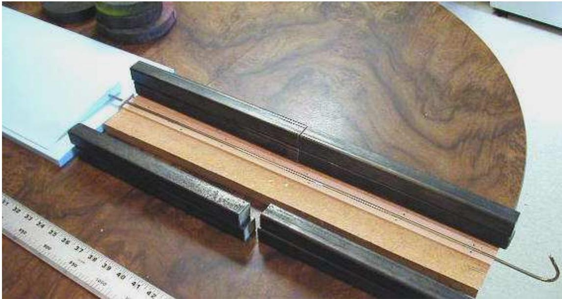
At the front of the board, I screwed a plate of 1/8" aluminum in which I'd drilled a 13/64" hole. The hole was vertically positioned to put the rod flush to the board.
