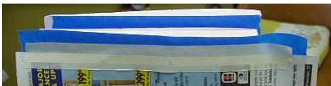
With the work angled, spray ends with 3M77. Remove masking. When tacky, progressively rejoin, working rearward keeping parts aligned in good contact to seal against bagging epoxy from entering & blocking the tunnel.
