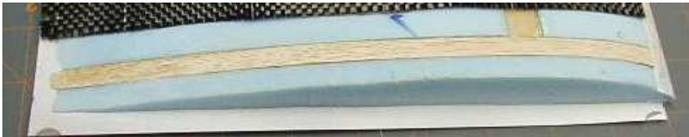
To size the top center carrier, place the .014" Mylar on the workbench. Lay the center core upright on it, core TE 1/4" ahead of a Mylar edge. Mark around the overcaps & LE. Cut the piece. Use it as a pattern to cut one with 1/8" less chord for the bottom. Mark ID on the outside of each carrier. With the core 1/4" ahead of carrier TE's, carriers will fit some over the glass taped LE but not touch.
