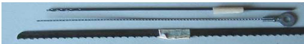
Pull plug pieces out with piece of coping saw or bandsaw blade, etc.
