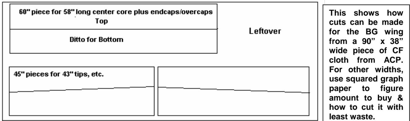
12" wide cloth is quite convenient to work with. Two times the span in one piece will do, but if it is \$1 cheaper per foot for 25', as with CST, get 25', spend less in total & have some extra cloth.
