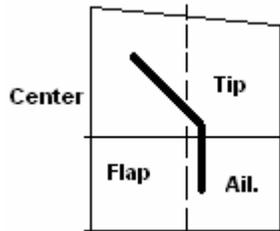
For the ROTARY DRIVER SYSTEM (RDS) inboard aileron chord must match outboard flap chord as depicted here.
