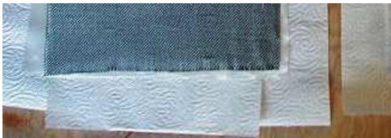
Not visible here, the painted bottom carrier is under the glass cloth under the CF cloth. To keep the bench free of epoxy, paper towel strips go under the carrier perimeter. Glass & CF cloth are wetted out at the same time. Then support carrier on finger tips to scissor off excess cloth. Toweling helps keep carriers clean for taping together.
