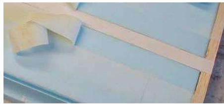
After sanding the fill smooth, remove the tape. Wrap 100 grit aluminum oxide sandpaper around a wood block. Level the spackle. During bagging, the Mylar will preserve the slight contour of the airfoil over the spar.
