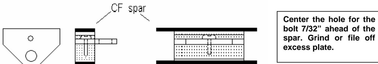
**BLADE BOXES:** Boxes are made as one-piece items to divide into inner & outer halves. In the drawing below, black denotes ply, gray the 1/8" x 3/8" spruce or bass uprights & white the balsa used only on the inboard half to make it spar width. Core Section 2 will be angled up relative to the outboard half to impart dihedral.
