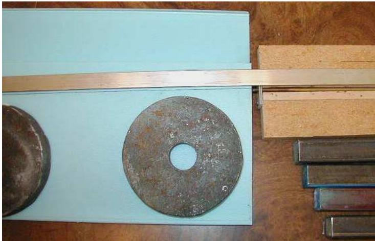
The objective is to tunnel about halfway into each piece from each end. Do one end of each, then rotate the bed 180 degrees to similarly do the other ends. Mark the rod about 8" from its front end to judge the halfway distance,
