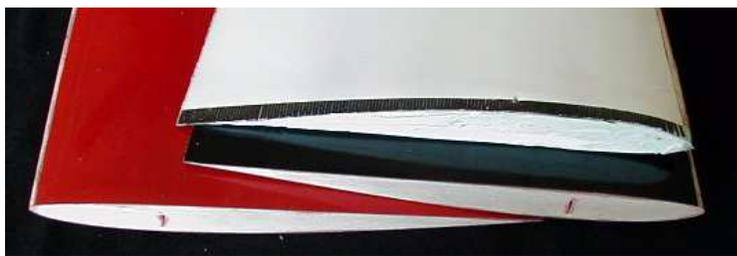
At top, the foam “overcap” is still intact. Carefully band saw off some. Dig out the rest to expose the carpet tape over the 1/64” ply cap on the endcap. Use the Dremel tool with sanding drum to trim almost to the 1/64” ply. Peel off the carpet tape. Finish with sanding block. Drill 1/16” holes through the balsa plugs defined with red marks.
