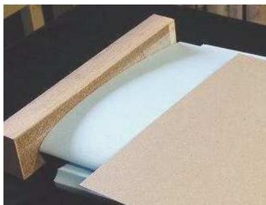
Go to the separate "INITIAL CORE PREPARATION" document. Do those steps & then return here. This pic shows how to square up core ends with a sanding block made as described in CONST. File 1.
