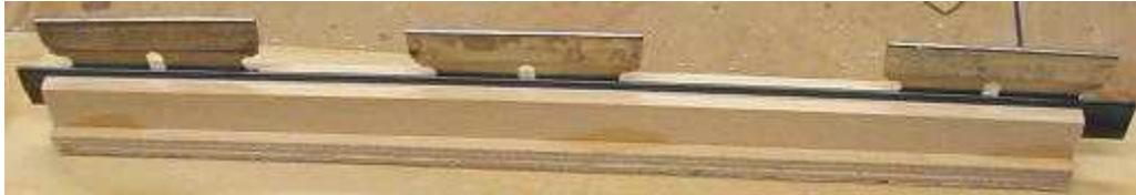
If using .050 blades, a waxed piece of 1/16" bar aluminum may be used for this step.
