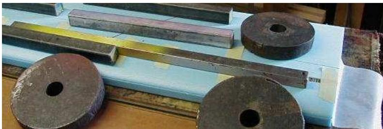
Bottom picture: Front cores are lastly attached using tape & weights to keep things in contact & down flush.
