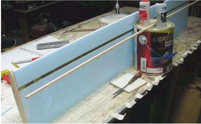
**ADDING LE'S:** Cut  $\frac{1}{4}$ " medium balsa, into  $\frac{3}{8}$ " strips. Bevel tops 25 degrees. 2 strips butted at the center are fine. Use quick epoxy to attach one at a time. Apply a light coat to the core. Wipe away excess at the top or bottom. Tape strip in place.
