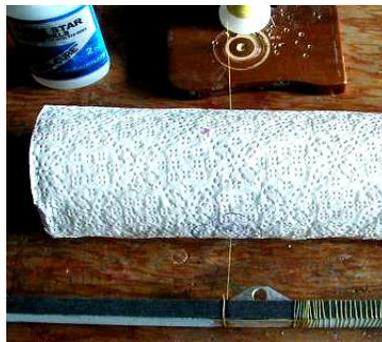
**KEVLAR THREAD WRAPS:** Sand sharp edges of the spars to blunt them. Tape a roll of tape, etc. upright to the bench to support spar end as you wrap the other side. Set dowel in a board as a spindle for the spool. For tension, run a weight (lead shot filled steel tube, etc.) into a paper towel or toilet tissue roll. Lay roll on the thread. Tack thread to spar well with CA to rotate spar forward. It takes 10-15 min. to wrap a side this way.
