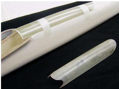
Using a razor plane, Stanley trimming plane & sanding blocks, shape the CCB down to merge to the nose block, canopy & SS edges. Finished results can be as seen below.
