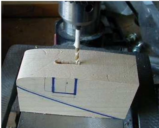
For slotting a 1-piece nose block, trim the bottom contour. Position block to make a series of uniform depth holes. Work the slot back & forth on the bit. Wax the tooth, insert it nicely squared up & fill around it with epoxy reinforced with Fillit, etc. to make a snug fitting slot.
