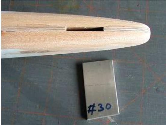
**3-PC BLOCK:** 1/8" ply can be used for the nose core. Add cheeks to the core. If you get a tight fit, the aluminum piece will stay put in the slot but be removable. If the ply is thicker than the aluminum, sand it down or wax the aluminum & fill around it with thin ply or epoxy to get a snug fit.
