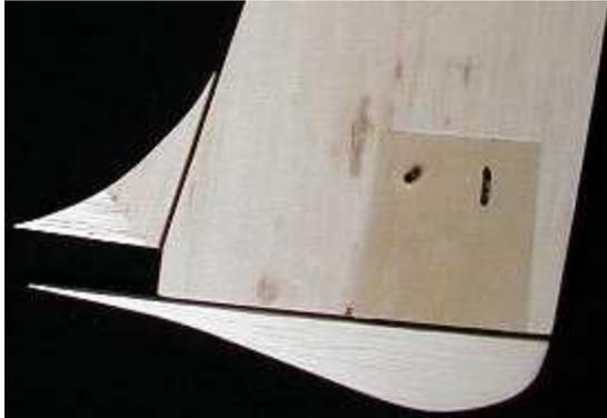
This skid, a 3-layer item, extends back in a nice curve from the front of the dorsal. The bottom 1/2" of the center layer is 1/8" ply. The remainder of the center layer & the outer layers are very light 1/8" balsa. The sides of the skid are tapered in a straight line down to the ply. The remainder is smoothed & filleted to fuselage contours with light spackle.
