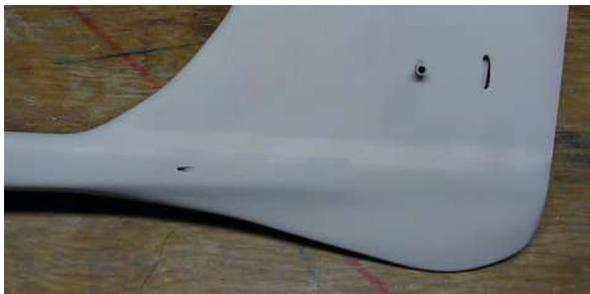
The top pic here shows the tail end after glassing over & priming. Note the rudder cable exit.
