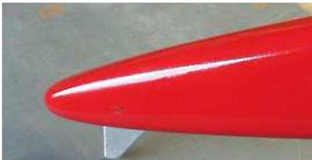
A 1/8" dowel pin secures the removable tooth, but will shear landing on concrete, etc. to help avoid enlarging the slot. A little hardwood wedge will close an enlarged slot.
