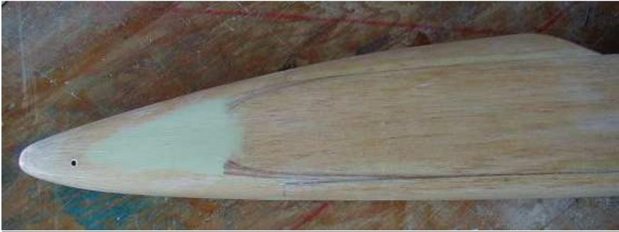
Note how the nose block, sides, closed compartment & fuse bottom all merge together for nice appearance. Icing putty fills beyond where sides end. Hole is where 1/8" dowel goes through to secure the nose tooth.
