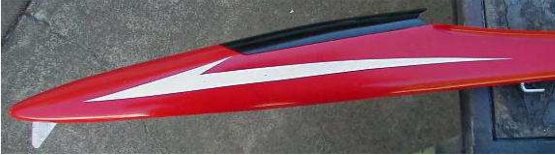
1.4-1.5 oz. plain weave glass cloth can be used overall, but using .5-.75 on the fin will keep it lighter & reduce nose weight needed to balance out. What follows assumes you've filled dings, cracks, contoured fillets & fine sanded overall.
