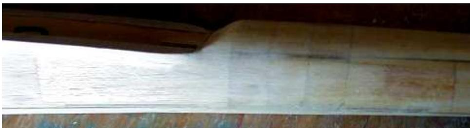
This shows a spiral reinforcing wrap of nylon tape over the full tripler of 1/16" balsa between 1/8" balsa doublers.
