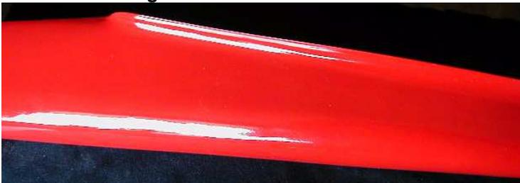
The pic shows the Rustoleum Gloss Protective Enamel before any waxing, polishing or buffing. It takes many days to cure to maximum hardness. **SADDLE AREAS:** to avoid wing & saddle paint rubbing, apply a heavier clear tape, such as book tape, on the saddle.
