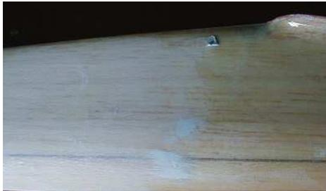
Left area shows the cloth brushed on with resin & block sanded dry with #80 grit. On the right the resin has not yet been sanded. All the shine is to be removed so the next coat will stick.
