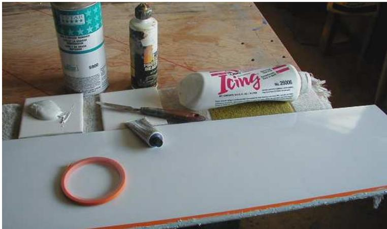
The top side of a GENIE #29 center is shown. The low tack vinyl tape gives a line to feather the putty to. Paper can be attached behind the vinyl with 3/4" masking tape for complete protection of the finished, bagged on paint. To minimize the chance of lifting paint when removing the tape, gently warm it with a heat gun. Too much heat will bubble the paint. The plastic bottle contains acetone to clean uncured Icing off the tile & spatula.
