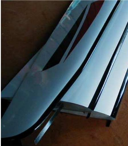
Left shows the first Big Smoothie high gloss panels by window light. The other is an SGP tip. Red & black swooshes go on the carrier inside first & that masking removed. Overall white is then applied before bagging.
