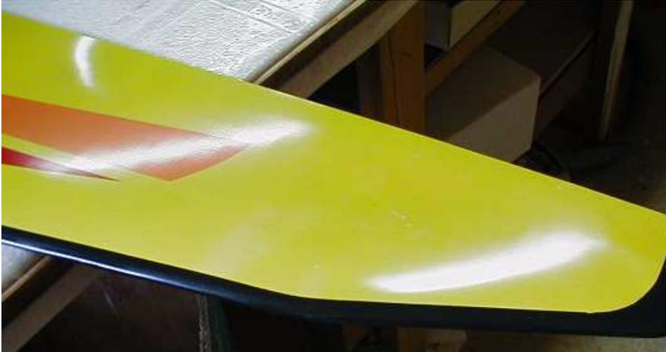
This shows a black LE trim. The red & orange swooshes are sprayed on the carriers before the overall yellow is applied. Masking ridges are flattened during bagging.
