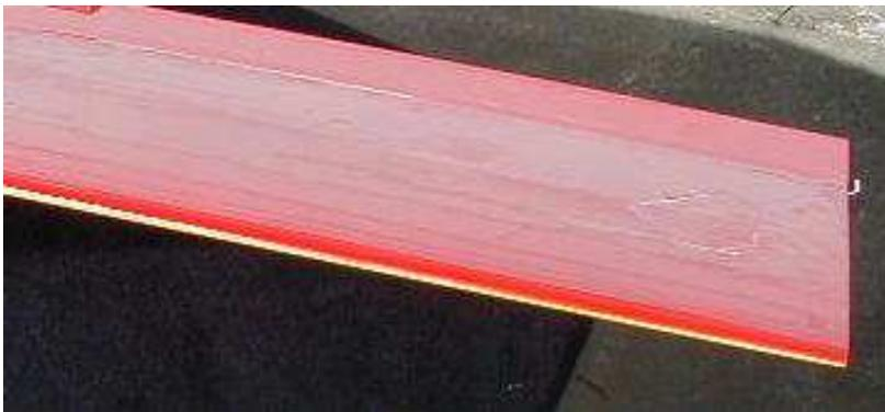
If using an overall paint when bagging that'll be durable on the LE, you can position a carrier near the LE to fog forward over it without fine line masking. Apply paint ½ or more around the LE on one side. Let it set up, invert & do the other side. If different colors, you get a 2-tone LE.
