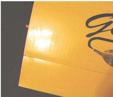
This is a unidirectional CF with bonded-in fray control filaments at 1/4" spacing to greatly simplify cloth handling. The pic shows the pattern of the filaments with 1.4 oz. glass placed first against the painted carriers. The 24" width provides a wing top & bottom with a 5" strip left over. Two such strips can be laid s/b/s for another top or bottom.
