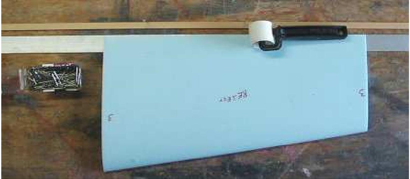
**This setup angles & guides the wall paper seamer roller to thinly compress the core along its extreme TE. Bear the roller against the guide & the work surface. Hold the core in place as you run the roller along the TE. Easy does it.**
