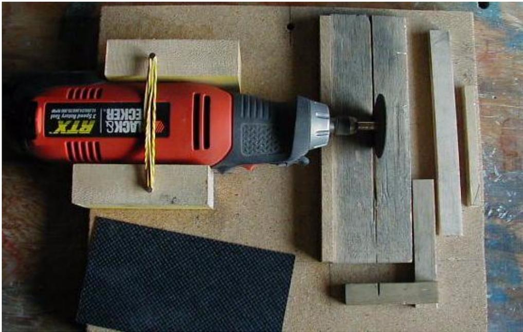
Use a heavier duty 1-1/4" disk. Blocks are glued to a base between which the tool is snugly secured. Rubber bands over the top work but a screw down plate or bracket would be better.
