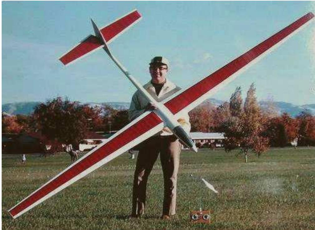
The Miskeet didn't do anything anywhere near as well as the GENIE, but got a lot of press way back then. According to an analysis by a 1970's aeronautical engineer-modeler it had the best L/D (27 to 1) of any contemporary R/C design. Well, it was hard to get down, that's for sure.
