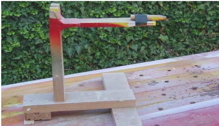
Pedestal snugly jams between the slab sides and serves as a handle while painting various areas of the fuselage. Top is slotted to fit around the stab pushrod. The taped-on dowel became obsolete when a slot in the former was later used in place of a hole. The slot allows easy pushrod adjustments. Ironing board comes in real handy for painting outdoors. Hunk of steel on the pedestal keeps it anchored in case a wind comes up.
