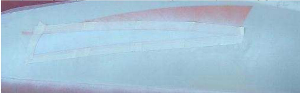
As shown below, with masking removed the carrier is sprayed yellow overall. This shows as the finish with the swooshes on top of it. Not shown here, white top coat is sprayed over the yellow to complete the pre-bagging painting. The white backing gives more brilliance to finished color coats that end up on top. White primer will crack and looks like a dry lake bed that shows through the finished color coats.
