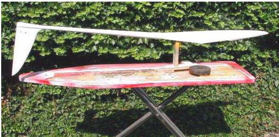
My 150" MISKEET (next page) appeared on the cover of the July, 1969 issue of FM and was the featured construction article. Huge stab was influenced by free flight design. The ship was later refined with spoilers, small stab and kitted by Ralph White (Fliteglas Laminates). It came in ready to fly at 64 oz. It had a 2-piece fiberglass fuse with circular cross sections that telescoped together behind the wing, making it easy to ship and get the tail aligned.
