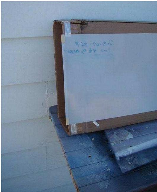
The 54" center section carriers for the Smooth Genie Pro can be secured with masking tape bits to a 48" box if the ends are opened and taped to extend the length. Fold the inner ends of the masking tape to easily peel it away but do not pull it inward or it will take paint with it.
