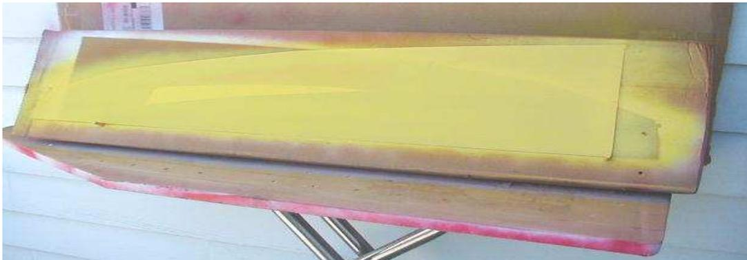
This is a different tip, all finished. Under vacuum, swoosh edges are flattened. Note close fit where tip butts center. This is possible with careful preparation of the endcaps, uniform application of the glass
