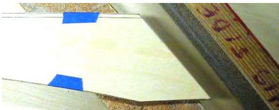
With sections taped together, bear them on one sanding block & true up the splice lines with another block.
