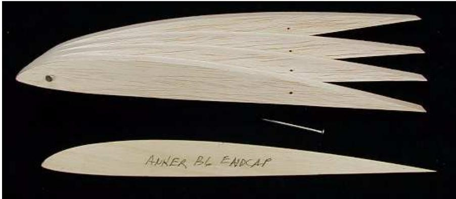
For endcaps, a ply pattern was made where core Sections 1 & 2 butt. Four blanks were cut from 1/2" hard balsa & the top one marked for stack cutting with the bandsaw. 2" brads kept the pieces aligned. The stack was finished with a disk sander. After slotting for the blades & beveling to 3/8" & for dihedral, etc. they are glued on.
