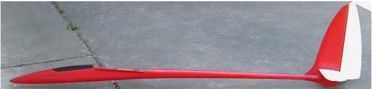
There are several differences between this ship & the regular Big Genie. For the wing spar I abandoned  $\frac{1}{2}$ " wide CF spars. Instead I went for  $\frac{3}{8}$ " using a double tapered one on the top only & .045" non-tapered on the bottom. That reduced weight & cost per wing although I had to buy pairs of each from ACP. The vertical tail is the full size one on the plans. The liberal “Vertical Tail Volume Coefficient” means even smoother, more solid tracking.
