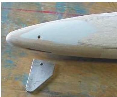
A nose block, drilled out & filled with lead shot/resin mix, is glued in 1" between the sides. Balancing out should be easy unless you get the tail too heavy.
