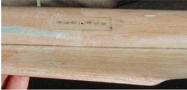
Balsa over 1/64" ply sub-decking is shaped top & bottom. Here, the exterior towhook blocking is seen. The saddle is filleted & contoured using 3/8" triangular stock. The continuous dark line is the sub-decking edge. It forms a reference line to sand to when shaping the fuselage.
