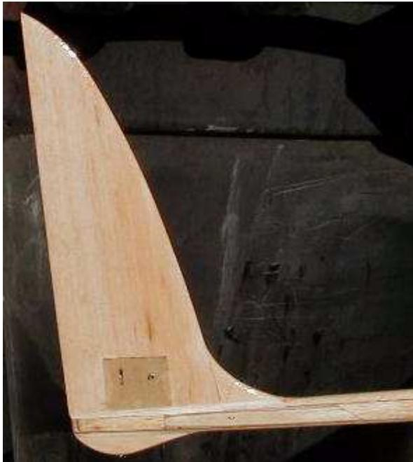
The fin mounts directly between the slab sides after the bellcrank has been installed.
