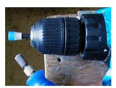
To reduce coupler bulk and weight for DLG's, use the setup shown here to sand it down, first reducing overall diameter, then taper smaller to the hex end. Reduce length by 1/8".
