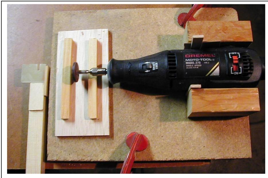
To a  $\frac{3}{4}$ " base, glue a  $\frac{1}{4}$ " thick platform. Snugly support the Dremel between glued-on blocks. Stabilize with shims or attach a metal strap over it. Optionally, blocks can also be glued either side up front to further stabilize it. Note the tool can still be shifted laterally. This enables positioning the cutting disk in
