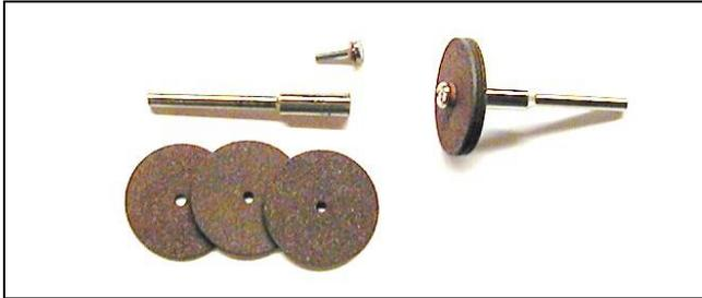
Tightly attach the disks on a mandrel with the little fiber washer under the screw head. If needed, clamp disks to make flush contact. Wick thin CA glue around the perimeter. Let it cure well.
