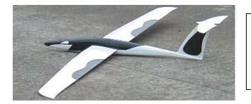
The '89 version TE sweep looked racy, but extra area behind the wing pivot point made hard work for the servos at higher speeds.
