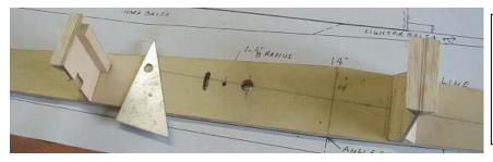
Glue triangular stock (TS) to the front of F1 & both sides of F2. Attach servo rail to F1. With the right SS down flat, glue on formers, upright.
