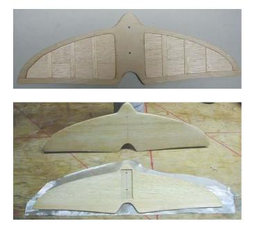
The top picture shows the 1/32" ply core glued to the 1/8" bottom, edges trimmed to core. Next, the 1/8" top has been glued on, & all surfaces gently rounded, ready for glassing-over. To top side, brush glass down smoothly & wrap it around the edge & over the bottom a little. Sop excess resin. Let this cure, sand bottom glass edges smooth, & then size a glass piece to fit the bottom & brush it down. Sop excess. When cured, sand the overlaps smooth.
