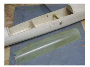
Trim the glass canopy to its molded-in reference lines. Out of the mold, it may widen or narrow. Make pliable with heat gun. Squeeze between blocks to narrow. Press to widen. The 1/8" balsa fuse doublers are <u>contoured to SS outer edges to make oval-like</u> <u>cross sections along entire fuse.</u> Tape canopy in place. Merge fuse lines to it. On balsa sheet, mark inside canopy to outline end supports. Cut & glue on as this pic illustrates.
