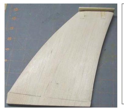
Later, after mostly shaping the fuselage, sand fin areas above the SS top edges to sort of a generic, symmetrical airfoil without flat spots. From a layer of 1/16" balsa & 1/16" ply, make the platform with bolt holes aligned to the brass inserts. Epoxy platform in place, squared-up, balsa side down. Strength & rigidity are later imparted in filleting & glassing-over. The bass stab blocks referred to below can be seen installed at the top of the fin under the stab platform.
