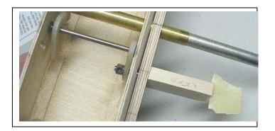
Measure how much pin should protrude to eliminate play between endcap & fuselage. Accordingly, glue pin into the block. Glue block into the core. Fill over & under it as needed.
