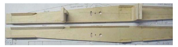
Forward of the fin, the TS is to be trimmed to allow clamping it between the SS's. Preferably, use solid 5/16" very light sheet balsa for the fin. 3/8" is overkill.  $\frac{1}{4}$ " is too thin for the threaded inserts. Alternatively with 3M77, laminate light 1/8" balsa sides to a 1/16" light balsa center.
