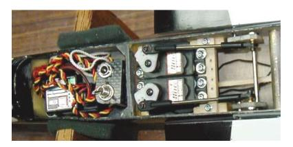
Wanting plenty of power for high speed, high wind work, Jay Decker did this installation with 150 oz. in. Hitec 5945 servos & Rocket City Missing Link fittings.
