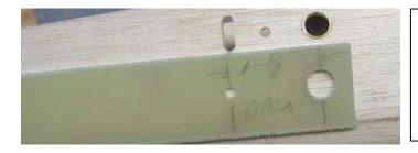
**DRIVE PIN SLOT GUIDE**: Run 11/32" tubing through the stacked sides. Make a guide as shown to drill a 3/8" arc-shaped opening. If more deflection is ever wanted, it can be extended with a 1/8" round file.
