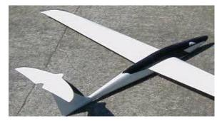
This new wing has equal LE & TE sweep. Pivoting at 45% of chord, the aerodynamic balancing makes lighter work for servos. The new Mark Drela airfoil combo optimizes overall performance & handling.
