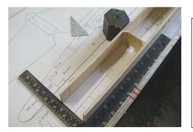
Review next picture about TS. To attach the fuse left side, position the work upright as shown here. Use a carpenter's square to align the front ends. Use weights or clamps to keep things together as glue dries. Keep flush to the workbench from 0" to 14" to align sides in profile. As shown below, preferably glue TS to the SS edges before joining them to the formers, but leave space on the left SS, as shown, to later fill in next to the TS on the formers.
