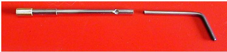
A silver solder that melts at low temperature is essential. Higher heat will oxidize wipers and SS tubes inside and out to prevent solder flow.
