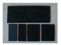
The slot inside surfaces should be rigid & durable. .028-.032" carbon plate is ideal. From a 1" x 2-1/2" piece, cut a pair  $\frac{1}{2}$ " wide & cut the remainder down the middle.
