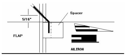
The shaft engages a slotted unit fitted between the aileron skins. A groove is to be made in the tip section endcap to allow the shaft to slip into the slot. For illustration, the profiles are exaggerated in the above drawing, <u>but do notice the top CF piece is a little ahead of the bottom piece. This allows beveling for down deflection after the aileron is cut loose.</u>
