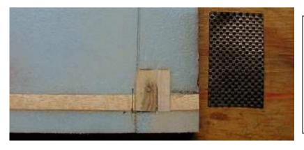
This shows the unit in the right tip of SGP # 4, ready to bag. Balsa fill has been shaped to the core. The foam overcap was divided to provide a reference where the inboard hingeline starts. A reinforcing layer of CF cloth goes over & under the aileron core before overall cloth is bagged on.
