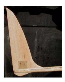
Here the fin with installed bellcrank assembly has been glued directly between the slab sides & filleted in with light spackle. Glass has been attached with a low viscosity epoxy. This is to be sanded down & a thin, overall 2<sup>nd</sup> coat applied to be wet sanded smooth. A filler/primer is applied & wet sanded glass smooth for painting.
