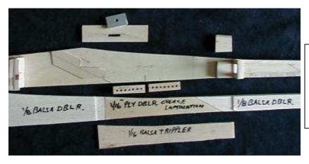
This shows the <u>inside</u> of the right SS & <u>outside</u> of the left. The left side displays the 1/16" ply doubler over CF laminate. After it is attached, exterior 1/8" balsa doublers are fitted <u>flush</u> to its ends. Attach them with a very thin coat of epoxy.
