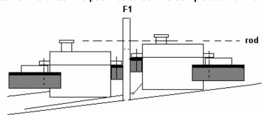
SERVO LOCATION: Servos need to be squatter micros such as the JR micros or Airt. 94761 to allow low routing of the stab pushrod & rudder cables. Former F1 locations shown on the SS patterns set servo locations.
