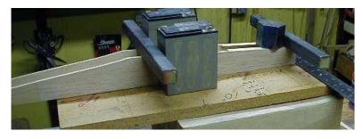
Use whatever's handy to keep front ends butted to the carpenter's square, sides upright & bottoms flush to the board. Do keep sides parallel until the glue is dry. Then pull together to attach narrower F2 & the other deep rail.
