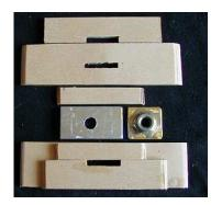
Drill a centered hole in the aluminum plate. If uncertain about tapped thread strength, solder a nut to a plate of thin brass. Secure it to the aluminum plate bottom with adhesive or screws. Cut 1" x 4" side plates from 5 ply, 1/8" ply. Use 1/8" drill bit & flat file to make <a href="mailto:snug">snug</a> slots ½" down from the top. Glue 2" x 3/8" bottom strips in place for <a href="mailto:snug">snug</a> fit to the aluminum plate, so the unit will be squared-up & stand alone, nut pointing down.
