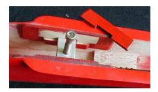
MOUNTING THE UNIT: Less the notched pieces, bolt the unit to the wing. Position the wing on the saddle. Squeeze fuselage & remove the wing. Mark unit's location. Use a strong wood glue such as Elmer's Ultimate to glue it to the sides. From 1/8" ply, size pieces to jam fit front & rear between the 4" pieces to press them snugly to the sides. Let dry, then glue on the notched pieces to complete 1/4" deep recesses for the plate ends.
