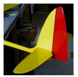
This is an LT/S tail end. On all ships, small cross section in this critical area includes CF laminate between ply doublers to minimize chance of breaking ahead of the fin. Light tail helps keep stress low on fuse in hard landings.
