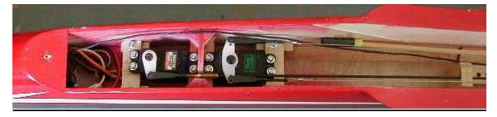
Extreme right, the front hole of the towhook block is visible. To its front edge a slotted block of ¼" balsa is glued upright & capped over as another pushrod guide & support. Front end of the stick
