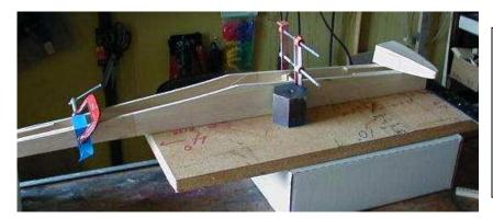
It's essential to butt both front ends flush to the carpenter's square to precisely align the sides to each other & to F1. See next pic.
