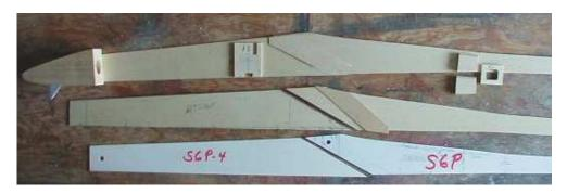
Pic shows nose block, formers, "deep rails" by rear former, SS's parts & splicing doublers. The white stuff is Sintra, about 1/32" thick.
