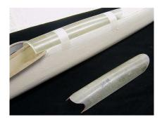
Rear end of the canopy is contoured to the actual mounted wing & ends up shaped as in the foreground. This rear end fitting is done in increments so it nicely fits around the LE. A "stop block" is glued to the inside of the fuselage to prevent the canopy from gouging the wing.
