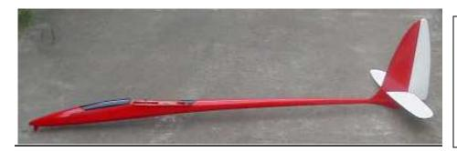
This is the longer, slimmer, Smooth Genie Pro/Big Smoothie fuse. Pictures don't do it justice. The ply slab sides on this one were cut with more bow between wing and tail as shown on the Aug., '09 plans.
