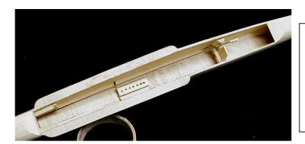
The internal part of the tow hook blocking glues to an internal 1/16" ply plate. ½" triangular stock is placed where SS's meet the bottom. The wing saddle is widened with 3/8" triangular stock & capped over with 1/64" ply. The solid CF pushrod passes through the supporting straws tube installed before the fuselage bottom is closed up.
