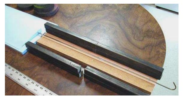
At the front of the board, I screwed a plate of 1/8" aluminum in which I'd drilled a 13/64" hole. The hole was vertically positioned to put the rod flush to the board.
