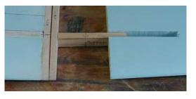
Slip a blade into the center section. Slip on the <u>tip</u> endcap. Slip on the outboard box <u>being sure it's</u> <u>not inverted</u>. Block up the other center section end 4 degrees. Blade here was ground to an angle & box bottom tapered to better clear the work bench. Center can be jacked up another degree if more dihedral is wanted for turning ability.
