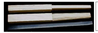
Undivided BG boxes for ½" spars once used are shown here. After dividing, outer halves are to be closely wrapped with Kevlar thread to prevent splitting out under launch stresses. Inner halves go between the CF spars before wrapping.
