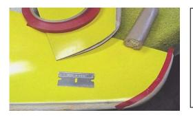
Knead a bit of the 2-part putty stick to judge working time available. Cut off a slice & roll it between palms to make a "worm" fatter in its middle. Press into the recess. Wet fingers with spit. Shape & contour putty to merge to skins. As it progressively cures it can be carved & wet sanded. It quickly hardens in the sun, ready to paint. If using darker trim paint on the putty, work in the shade. Paint on it will bubble in the sun.
