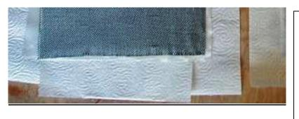
Not visible here, the painted bottom carrier is under the glass cloth under the CF cloth. To keep the bench free of epoxy, paper towel strips go under the carrier perimeter. Glass & CF cloth are wetted out at the same time. Then support carrier on finger tips to scissor off excess cloth. Toweling helps keep carriers clean for taping together.
