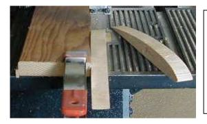
Here, with bandsaw table not tilted, a  $1/8" \times 3/8"$  strip (extreme left) has been attached to the edge of a 3-1/2" board to tilt it 1/8". The guides for the blade should be set to prevent blade wobble. Use a sharp blade or a straight line cannot be cut.
