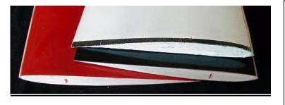
At top, the foam "overcap" is still intact. Carefully band saw off some. Dig out the rest to expose the carpet tape over the 1/64" ply cap on the endcap. Use the Dremel tool with sanding drum to trim almost to the 1/64" ply. Peel off the carpet tape. Finish with sanding block. Drill 1/16" holes through the balsa plugs defined with red marks.
