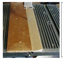
Little down aileron is needed for turn. TE camber for launch requires more. Tilt bandsaw table or tape a beveled support to it. Against the blade, clamp a board. Experiment with a 5/16" sq. strip of balsa to learn how to make the bevel. Bear the <u>inverted</u> aileron on the support & against the board to bevel it without taking anything off the top skin. Finish up with sanding blocks.
