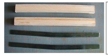
Initially, make these boxes with 1/8" thick tops & bottoms. Add to the <u>bottom</u> to get to web height. Mark which is the <u>top</u>. After dividing the box at its center, the <u>outboard</u> half along its <u>bottom</u> can be tapered toward its outboard end. See pics on pg. 8. When jacking up the center section to set dihedral between Sec. 1 & 2, this tapering optionally allows a bit more dihedral before the outer box end pokes out of Sec. 2.
