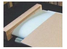
Go to the separate "INITIAL CORE PREPARATION" document. Do those steps & then return here. This pic shows how to square up core ends with a sanding block made as described in CONST. File 1.
