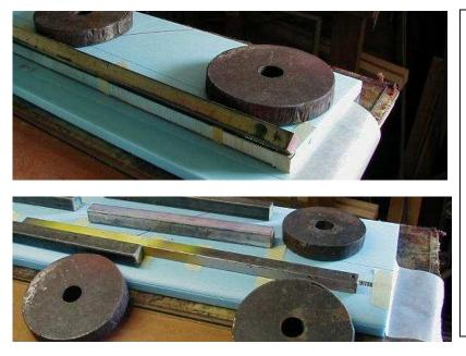
Separately first attach shimmed spar to core rears. Use masking tape & weights to keep it flush to core & beds <u>so no wrapped spar</u> <u>protrudes above the core.</u> Any bottom oozing will be flattened to the wax paper & not interfere with later spackling there.
