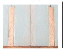
Centered 1-1/2" either side of the center line, remove foam to receive 3/8" x 3" balsa strips that match the airfoil. This makes the 3" wide extension between the flaps rigid. After bagging, cut to the hingeline with a razor saw replacement blade. Paint wood for nice finish.
