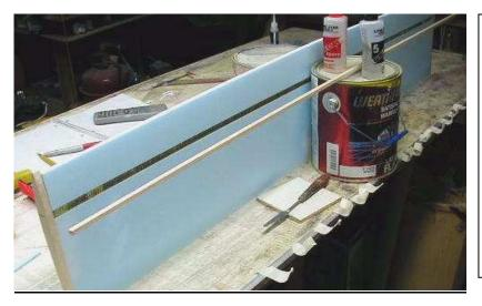
ADDING LE'S: Cut ¼" medium balsa, into 3/8" strips. Bevel tops 25 degrees. 2 strips butted at the center are fine. Use quick epoxy to attach one at a time. Apply a light coat to the core. Wipe away excess at the top or bottom. Tape strip in place.
