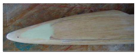
Note how the nose block, sides, closed compartment & fuse bottom all merge together for nice appearance. Icing putty fills beyond where sides end. Hole is where 1/8" dowel goes through to secure the nose tooth.
