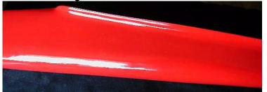
The pic shows the Rustoleum Gloss Protective Enamel before any waxing, polishing or buffing. It takes many days to cure to maximum hardness. <u>SADDLE</u> <u>AREAS</u>: to avoid wing & saddle paint rubbing, apply a heavier clear tape, such as book tape, on the saddle. WEIGHTS: Building #7, I had an excellent selection of wood in the recommended densities. Without any built-in nose lead, weights were as follows:
