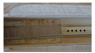
This shows front of the saddle caps and the interior portion of the towhook blocking. ½" triangular stock on either side secures it to the SS's & the 1/16" ply plate across the bottom of the fuselage. To keep spray paint off the pushrod it was covered with a straws. Masking tape goes against the fuse interior walls before painting so good glue joints can be made when installing the main bolt holddown unit.
