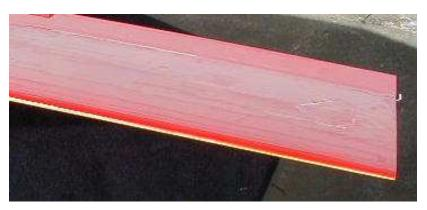
If using an overall paint when bagging that'll be durable on the LE, you can position a carrier near the LE to fog forward over it without fine line masking. Apply paint ½ or more around the LE on one side. Let it set up, invert & do the other side. If different colors, you get a 2-tone LE.
