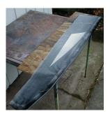
Outdoors, a card table supports a panel. Here, the top LE trim had first been done & that masking left intact while doing the masked bottom shown. Masking keeps overspray off the bagged-on paint. When the LE is painted, clean off any paint on your fingers. BEWARE: The paper has fresh paint on it. Get a clean hand under it to grab a panel. Utilize gravity to dangle loosened masking away from the new paint. Extra hands are very helpful when removing masking.
