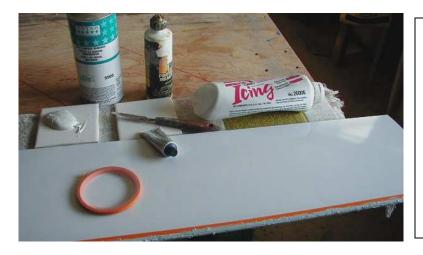
The top side of a GENIE #29 center is shown. The low tack vinyl tape gives a line to feather the putty to. Paper can be attached behind the vinyl with ¾" masking tape for complete protection of the finished, bagged on paint. To minimize the chance of lifting paint when removing the tape, gently warm it with a heat gun. Too much heat will bubble the paint. The plastic bottle contains acetone to clean uncured lcing off the tile & spatula.
