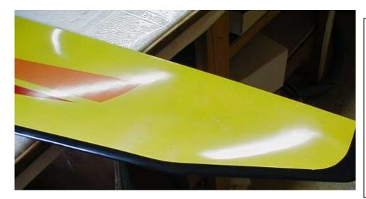
This shows a black LE trim. The red & orange swooshes are sprayed on the carriers before the overall yellow is applied. Masking ridges are flattened during bagging.
