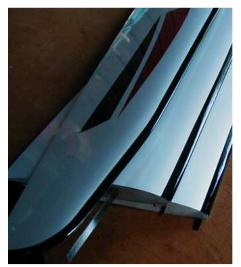
Left shows the first Big Smoothie high gloss panels by window light. The other is an SGP tip. Red & black swooshes go on the carrier inside first & that masking removed. Overall white is then applied before bagging.
