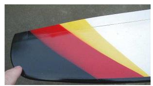
Multiple colors: Use a single, curved pattern cut from a manila folder or thin cardboard. First apply the lightest trim color inboard by fogging over the pattern held steady a bit above the surface. That makes a fairly fine line. After that's set, angle the pattern out a bit more to apply the next darker color, fogging over the edge toward the tip to minimize overspray on the prior lighter color, etc. When those are dry, mask to do the black LE.
