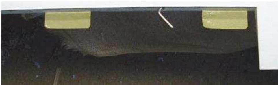
After slotting is finished glue hinges one by one on the wing side. When the glue is dry, protruding hinges & the flap drive shaft are slipped into the slots & the pocket.
