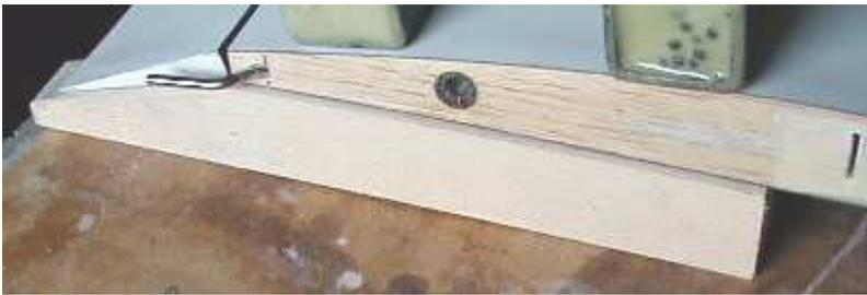
From  $\frac{3}{4}$ " wood, cut four 1" x 6" flap supports. Bevel the rear 2" at 20 degrees to keep flaps aligned to wing as the silicone cures. Note protruding drive shaft, the rear epoxy socket for a dowel keying pin & the blade slot.
