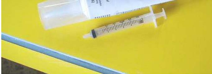
A small syringe without the needle makes a good applicator. Trim off any housing around the nozzle. Let the taped surface droop over the edge of the workbench.
