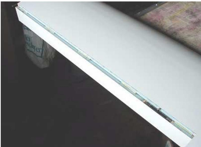
Here's a completed installation on an LT/S flap. Five hinges were used. One is inboard of the RDS pocket & another near the outboard end. The others are evenly spaced between.
