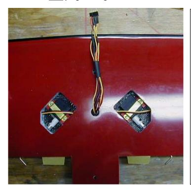
The male part of the connector is to extend a bit beyond the wing LE for handy connect & disconnect to the female (receiver) part of the harness.
