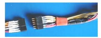
The wrap is a non-tacky electronic insulating tape that bonds only to itself & keeps all wires bundled.
