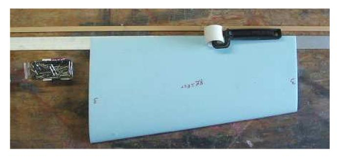
This setup angles & guides the wall paper seamer roller to thinly compress the core along its extreme TE. Bear the roller against the guide & the work surface. Hold the core in place as you run the roller along the TE. Easy does it.
