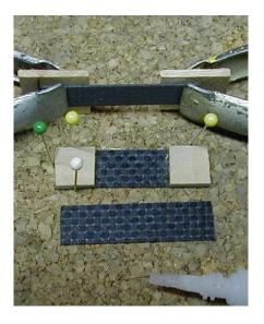
Wrap pocket ends with a single layer of fine thread, preferably Kevlar. It's essential that top and bottom stay in parallel planes during installation, neither bulging in or out. To assure this, prepare a waxed "insert" from spacer stock. Slip it in the opening. Over and under the pocket, fill with balsa shims and epoxy. Keep epoxy out of the slot. Keep all flat and straight until the epoxy has cured. Remove the insert
