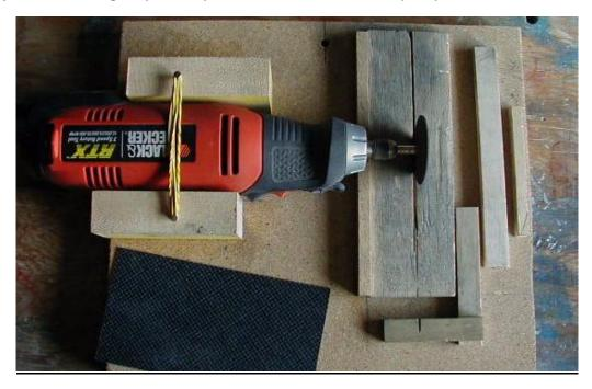
A rotary tool for cutting strips for tops and bottoms can be set up as pictured below.
