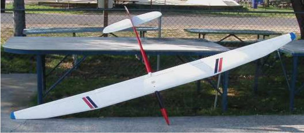
After losing 1/8" of core for skins & another 1/16" for a servo mounting base & a "hat bracket" as used on the HEMS servo mounts, the remainder has to fully recess common 1/2" thick servos without a bulge. The venerable SD7032 airfoil, employed on the very successful Jouster series of thermal competition ships & on early Big Genies, allows that. Tip cores are cut single taper & then, as explained below, are trimmed to create the planform shown above.
