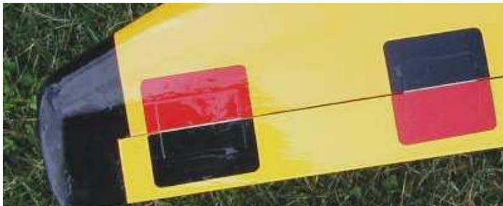
To hide the ugly Kevlar & make a decorative pattern, the hinges can be sealed over with either matching or contrasting 3/4" x 2" pieces of film ironed separately either side of the hingeline. The thin line of Kevlar showing can be hidden with a colored pen if you like. If a hinge lifts, reactivate the adhesive with a sealing iron or heat to peel off & replace.
