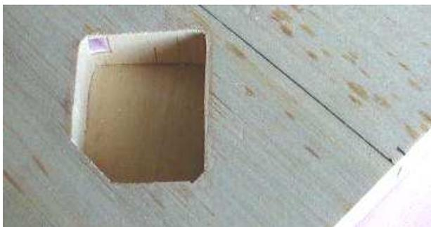
Here's a routed out aileron servo well reinforced with a plate of 1/32" ply & then lined with balsa to stick the film covering to. The black line represents the rear edge of the spar. The channel for the long servo lead is centered 1-1/4" behind the spar. Make aileron servo wells 1/4" shorter than for flap servos by jamming a 1/4" shim inside the template (File 3). Shift the template back 1/4" along the shaft path so the lead exits conveniently as shown here.
