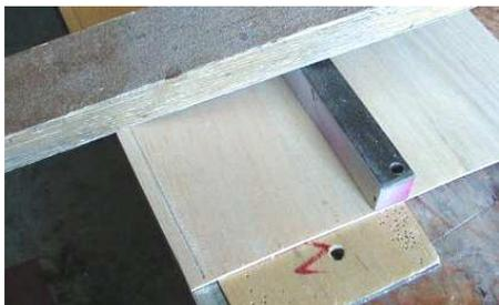
A zero thickness balsa TE is impractical. Using the setup shown, bevel both skin TE's inside close to zero. With a strip of 1/64" ply between them & a little outside sanding after skinning you get a thin, but practical TE. Up front, about 1/2" of wing will extend ahead of the fuselage high point for the canopy to fit around.
