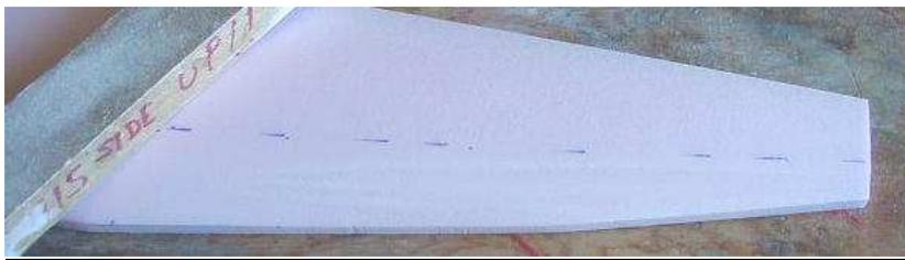
**MODIFYING THE AIRFOIL:** Use a 10"-12" long sanding block to gently shape the upper side to a generic airfoil without compound curves so the sheeting will lay flush to the core.
