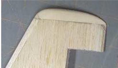
To tip sections add top skin, LE & tip block. A small block of bass, etc. can be shaped & flush glued to the squared-up extreme tip. Cut the aileron loose. Note the 1/64" ply between the skins at the TE.
