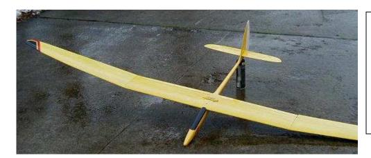
The composite fuse, shown here, is longer behind the wing. Handling is smoother in the pitch axis. The August, '09 plans show a 2-pc. SS pattern this length for the glassed-over fuselage. Cut from a 48" ply sheet, it requires a splice up front like the SGP fuse.
