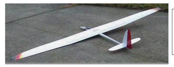
The LT/S can be built with one-pc. SS's cut from a 48" ply sheet & looks like this. Just shorten the pattern at the tail end as indicated for the Easy LT/S.
